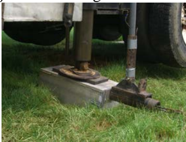
Figure 7: Seismic Pendulum Hammer Striking Aluminum Block with Rubber Pad Focusing Energy into the Ground
