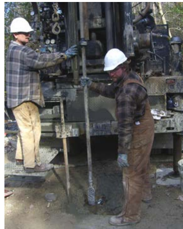
Figure 2: Lowering Torpedo DMT Blade into Borehole
