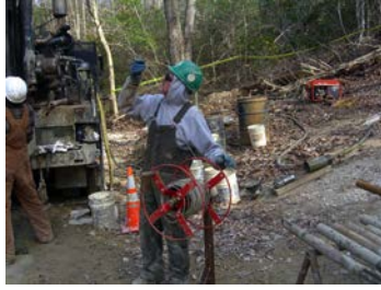
Figure 8: Reel to keep DMT cable from tangling
