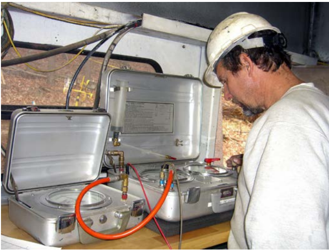
Figure 1: Standard Control with Auxiliary 100-bar Gauge
