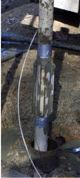
Figure 5: Taping DMT Cable to Outside of Rods Between Steel Centralizer Strips
